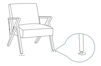
Attach 4 safety plugs (H) over the bolts as shown.
