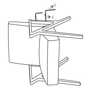
Attach 1 x back cushion to assembled frame as shown and secure with 2 x bolts (E). Tighten with an Allen Key (G).
